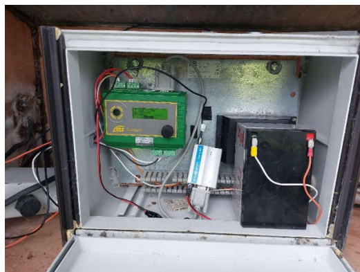
Plate 5: Aggard Bridge 29010 Data Logger
